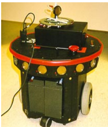
Figure 8: The Nomad Scout robot with the Polaroid ultrasonic sensor mounted on top.
